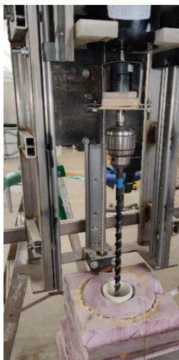
Figure 1: Drilling tests being conducted on cryogenic samples.
