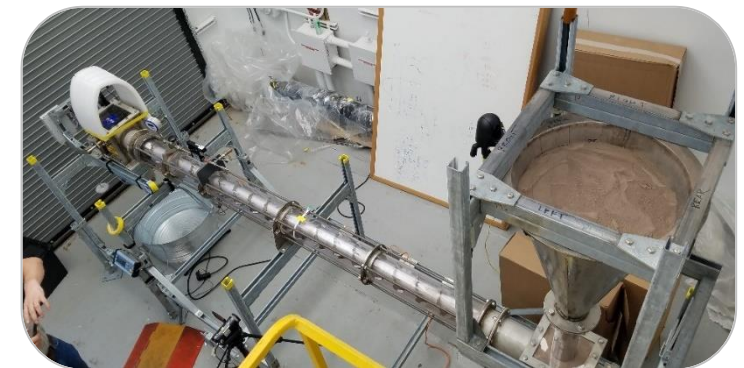
Auger Dryer for Water extraction Mars soil (ISRU)
