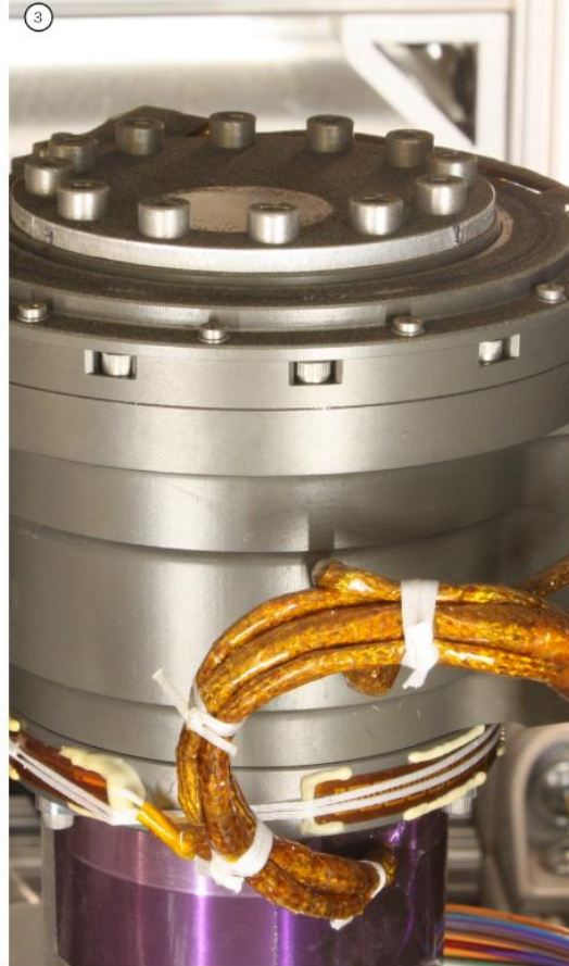
COLDArm Regolith Testing. (1) Test Venue (2) Actuator Output (3) Deposited Dust (4) Felt Seal
