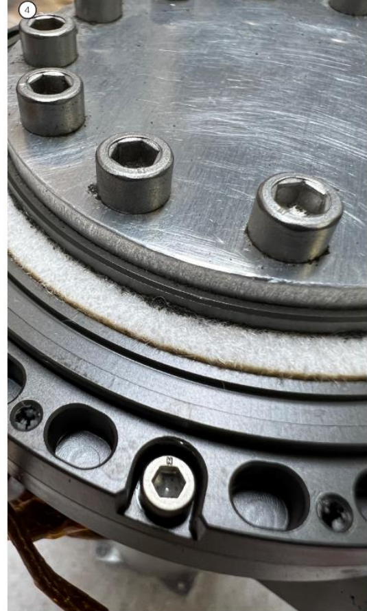
COLDArm Regolith Testing. (1) Test Venue (2) Actuator Output (3) Deposited Dust (4) Felt Seal
