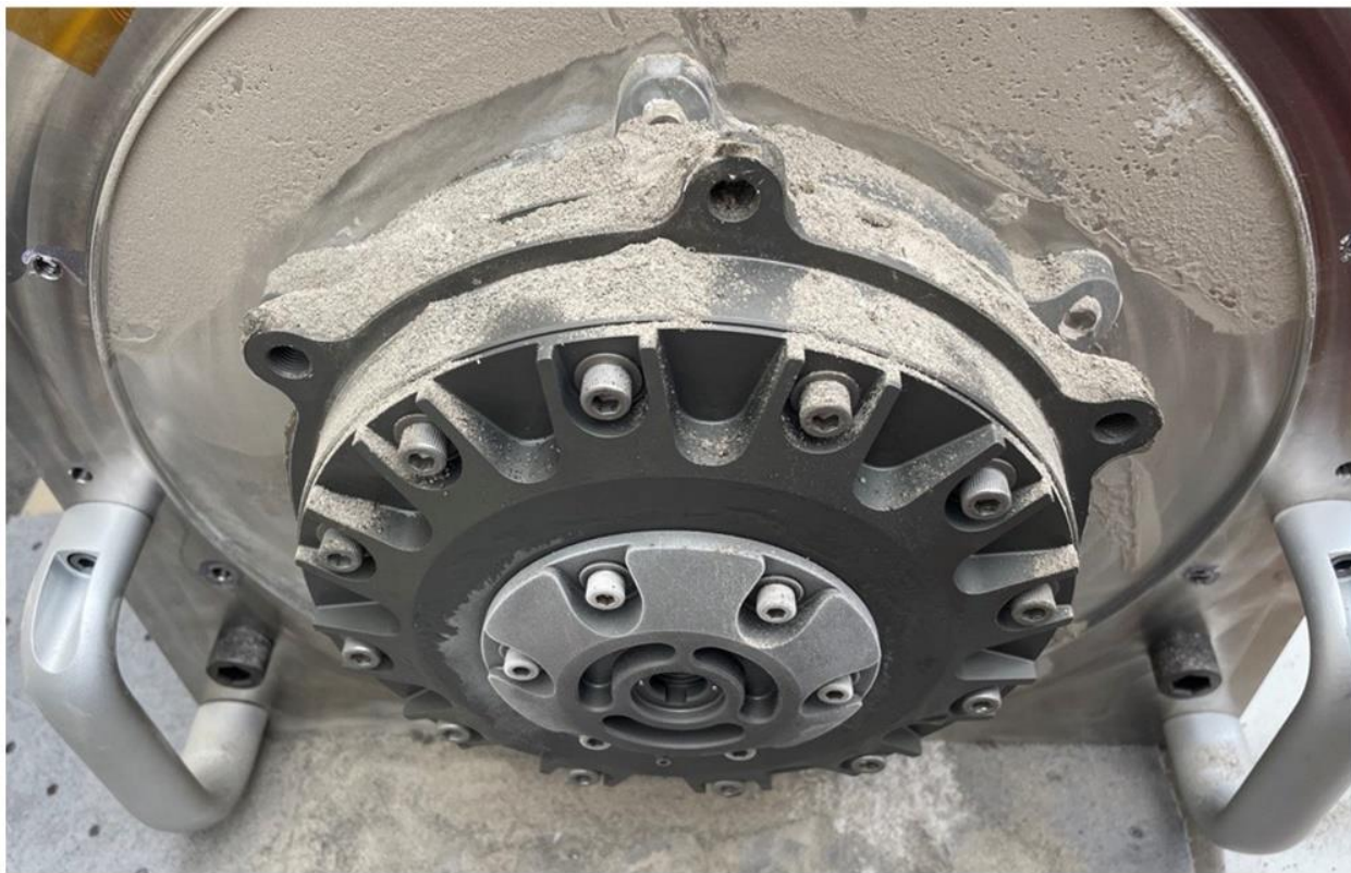
Regolith Life Testing on Motiv's LTV Actuator
