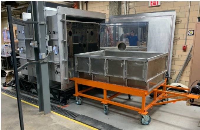
Photo of the new dusty thermal vacuum chamber
