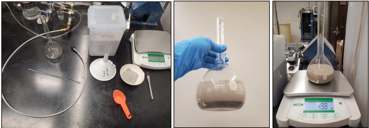
Figure 3: Lab set up used for Specific Gravity. (Left) The 500 mL volumetric flask, vacuum tube hose, thermometer, funnel, and scale used to conduct the experiment. (Middle) Simulant material combined with the water. (Right) Sample being weighed at the end of testing.
