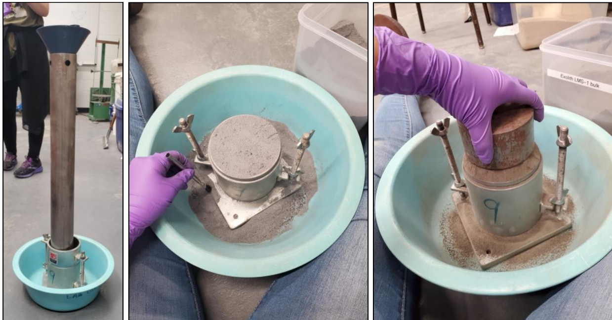
Figure 2: Lab set up used for measuring minimum and maximum density. (Left) Tube placed inside cylinder to pour regolith materials into cylinder. (Middle) Excess material being brushed off cylinder before measuring the final weight. (Right) Cylindrical weight being used to compact material into cylinder for maximum density measurements.
