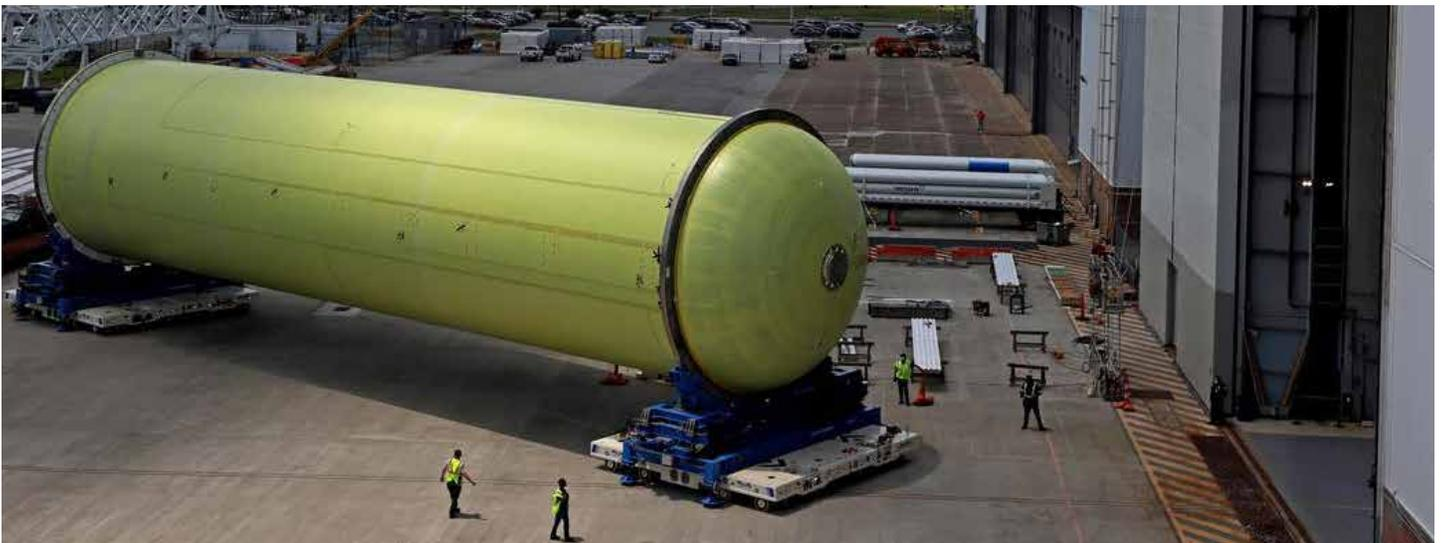
[MAF\\_20210429\\_CS2\\_LH2toVAB579](#): This image highlights the liquid hydrogen tank that will be used on the core stage of NASA's Space Launch System rocket for Artemis II, the first crewed mission of NASA's Artemis program. The tank is being built at NASA's Michoud Assembly Facility in New Orleans.
