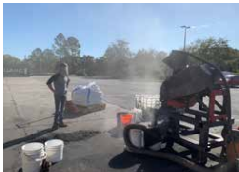
Simulant tech crushing lava rock with hammer mill
