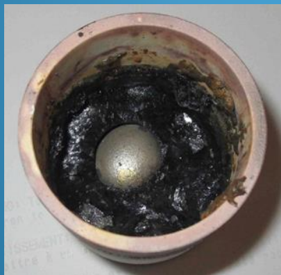
Iron Bead (from full melting in boron nitride crucible)
