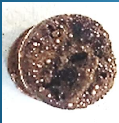
Initial Fe Coalescence (from high TiO 2 slag)
