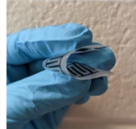
B CMrGO device fabricated on 3mil HDPE film
