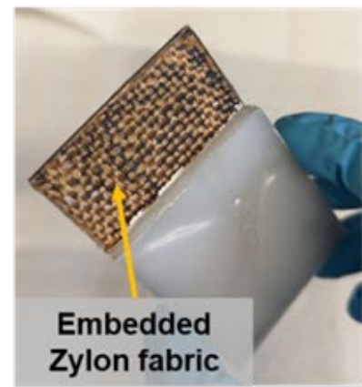
Zylon ® fabric embedded in a film of HDPE with a CMrGO infiltrated coating
