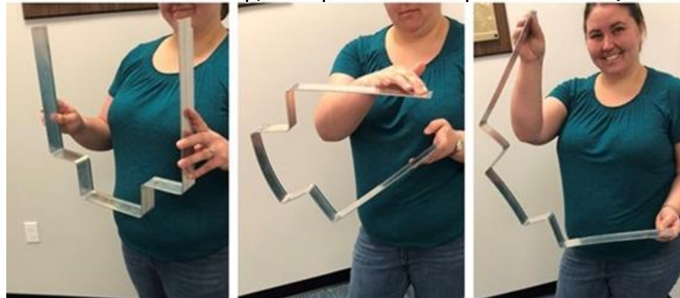
Flexible 1.2m OHP strap/transporter developed with AFRL/RV
