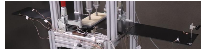
Updated heater clamping (bolted -> pneumatic) for improved contact uniformity and test repeatability
