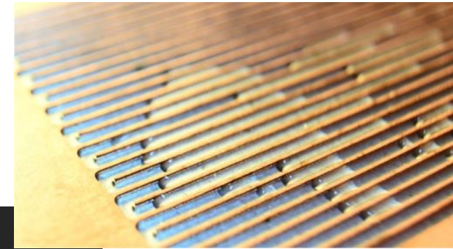
Photograph of CuMo OHP with liquid slugs and vapor bubbles (without lid)
