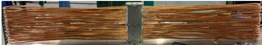
44" long copper bent tube OHP
