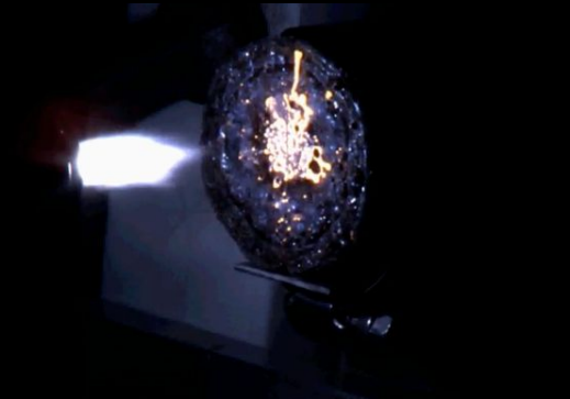
Figure: Plasma Torch Testing (3MW/m 2 )
