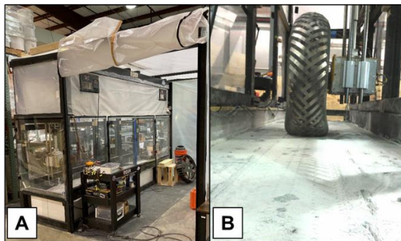
Figure 1. (A) The RIDER terramechanics testbed, including dust mitigation/containment features (sealed doors, airlock, air filters) and control station. (B) Replica Lunar Roving Vehicle (LRV) wheel being tested in RIDER as part of [2].
