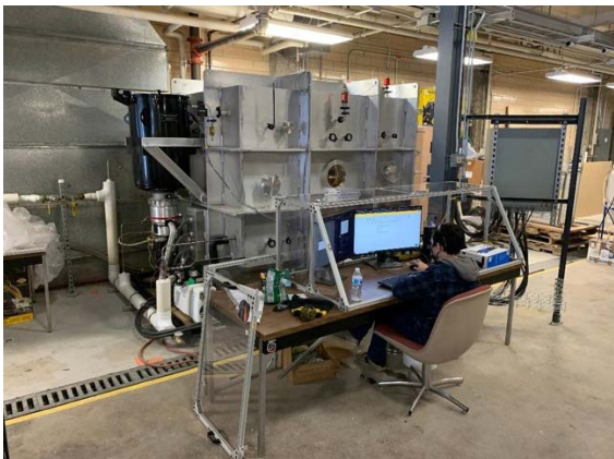
FIGURE 1. Existing Dusty Thermal Vacuum Chamber at Michigan Technological University’s Planetary Surface Technology Development Lab. Credit: Paul Van Susante.
