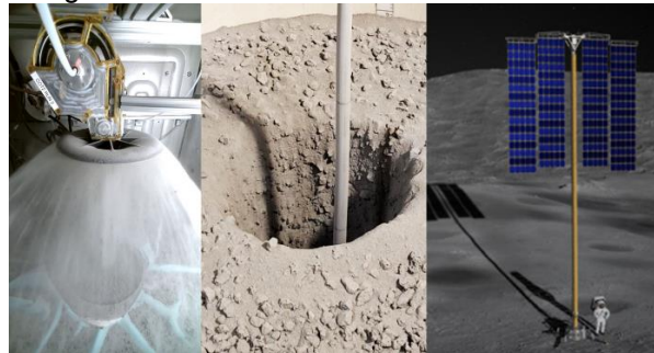
Figure 2. LISTER pneumatic drilling excavates a borehole of ~100 mm diameter to 3 m depth (right and center) DVF aims to capture these cuttings using the mast technology employed in LAMPS (right)
