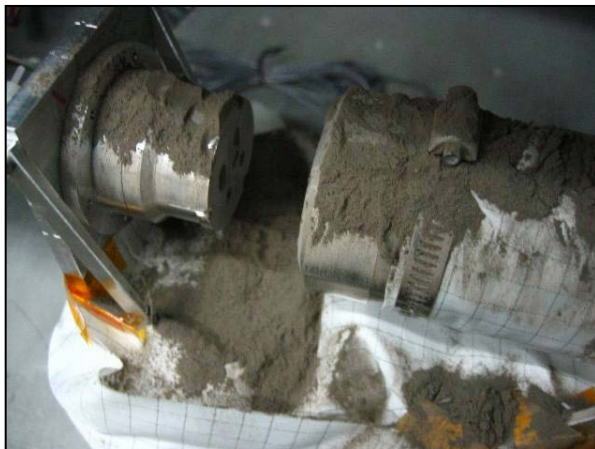
Figure 1. TRL 6 DTC undergoing dirty TVAC testing
