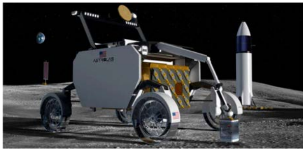
Figure 1: Lunar FLEX's modular payload interface and novel mobility system enables crew transport, robotic science, logistics, and infrastructure deployment
