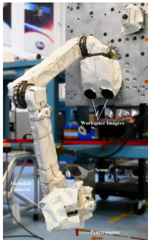
Figure 1: SAMPLR demonstrating a penetrometer plunge trajectory.
