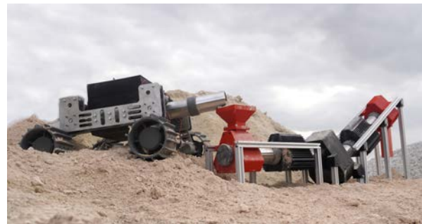
Figure 2. Rover equipped with an integrated modular drum conveyor, undergoing tests for regolith excavation and transloading to a fixed modular drum conveyor system.
