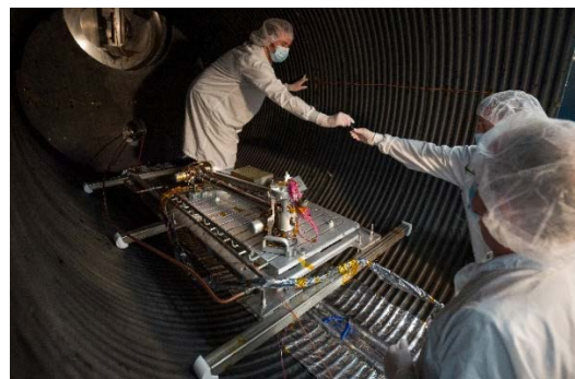
Figure 1: COLDArm system installation in 7 foot diameter thermal vacuum (TVAC) chamber at JPL
