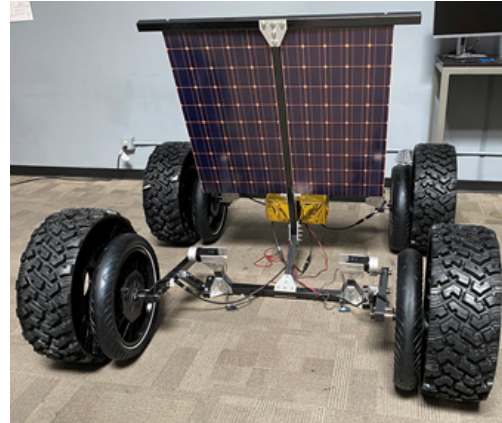
Figure 1- Maxar's Hybrid Iterative Testbed (HIT) for rover mobility technology evaluations.
