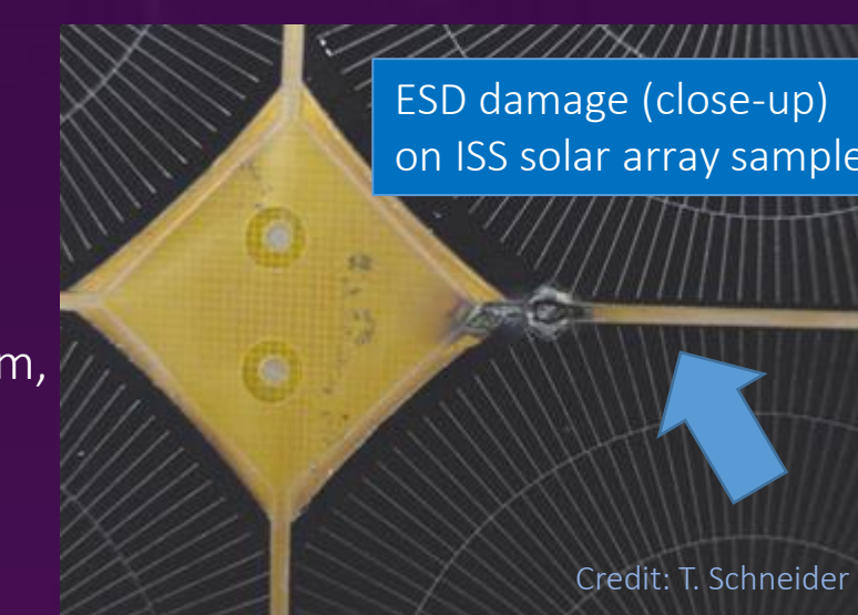
ESD damage on a European Space Agency satellite solar array
