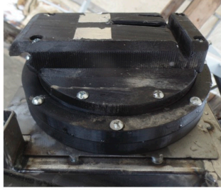
Heavily used 3D printed dual-pin tool coupler prototype, mounted on robotic excavator arm.
