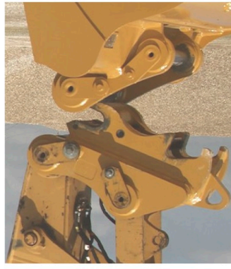
Our dual-pin system is a scaled down version of a quick-change excavator bucket attachment, like this Cat Pin Grabber (© 2021 Caterpillar), as widely used on construction sites for excavators between 10 and 100 tonnes.
