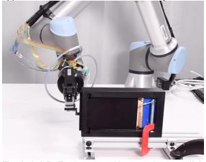
Fig. 2: A 6 DoF robot arm with a standard paralleljaw gripper is able to autonomously insert a module, mate its connectors, and lock it into place with the simple input motion of pivoting a lever.
